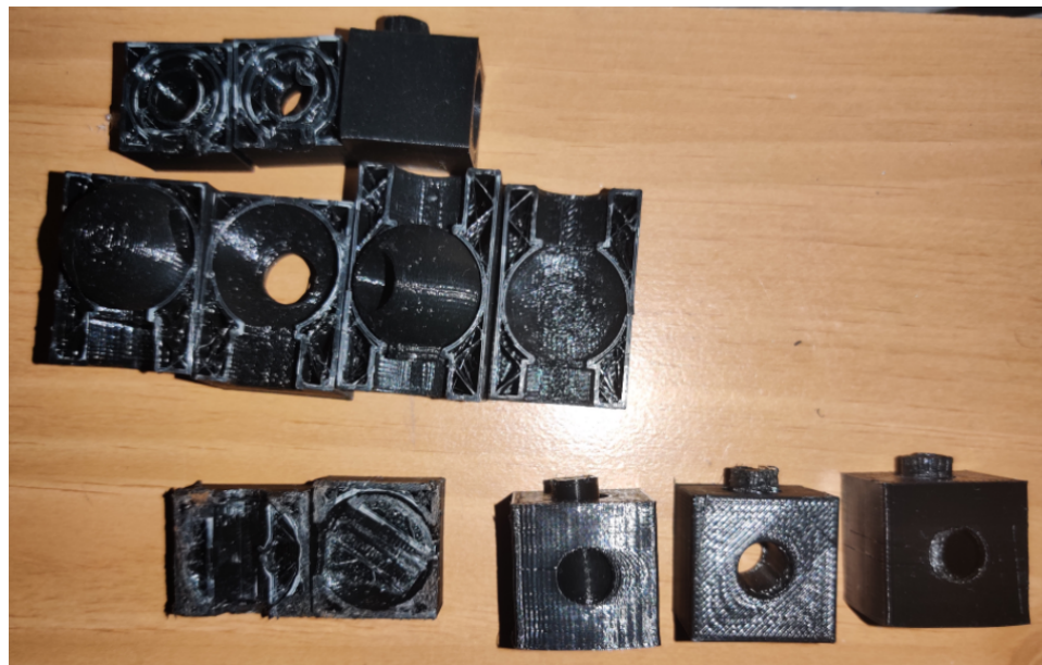
Figure 72: Iterative Design of Vent Ball Valves
